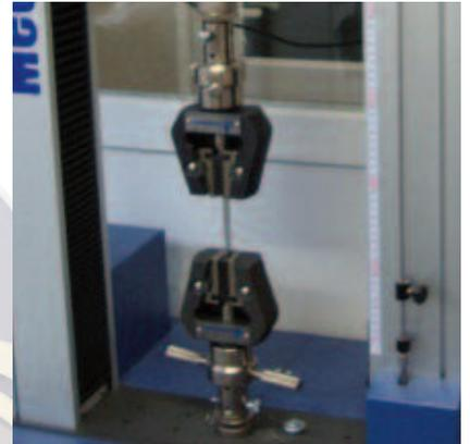
Tensile test on shutter material
